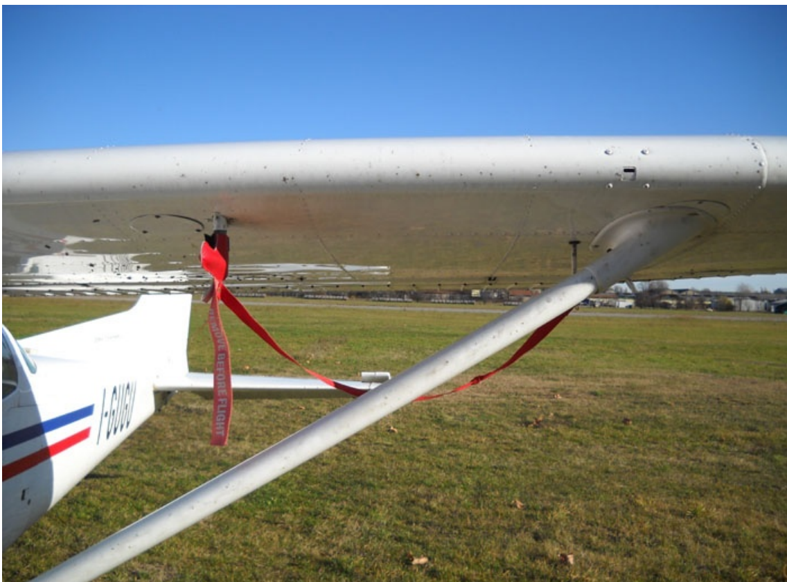
9- Pitot e fuel vent
